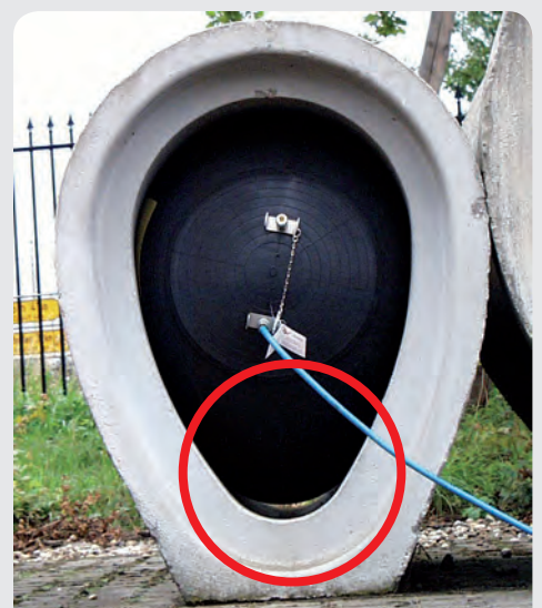
Egg profile pipe with round profile sealing bag - adaption problems, no sealing.
